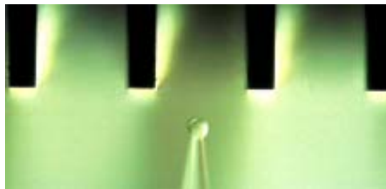
A close-up of the patch-clamped cell and the laminar flow zones at the microchannel outlets.
